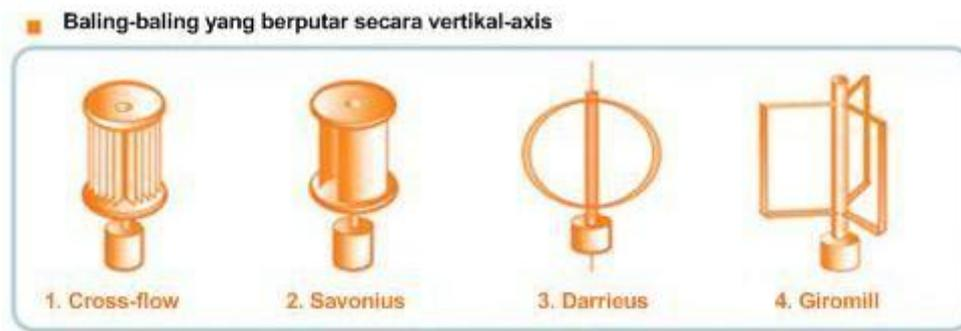
Gambar 2. Tipe Baling-Baling.
