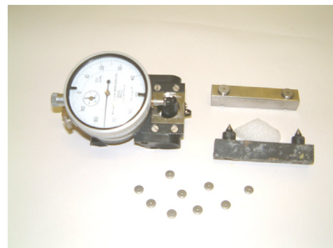
Figure 4. A Demec gauge, and its supporting equipment
