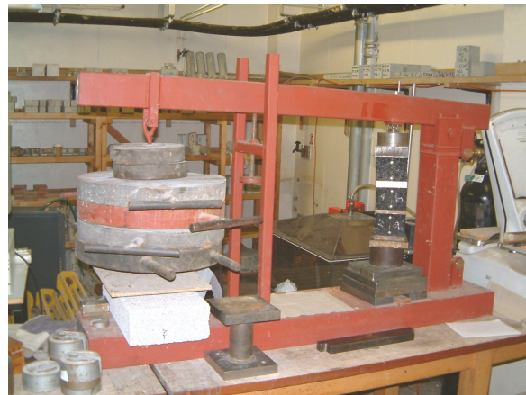
Figure 3. Creep test using a static dead-weight lever arm machine
