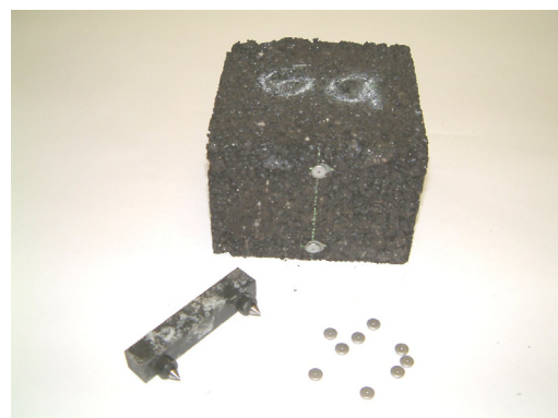
Figure 5. A sample with a pair of Demec points (dp) glued to its side
