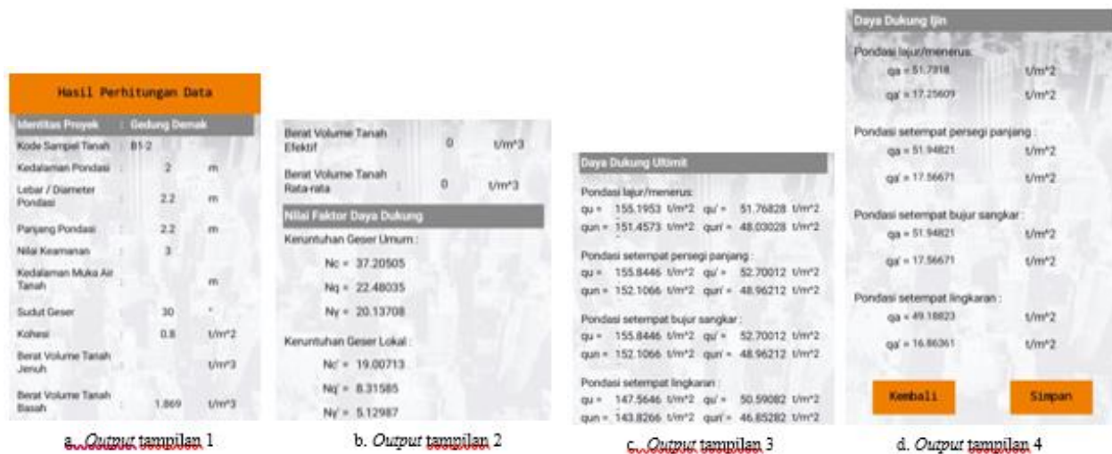
Gambar 10. Hasil Output Program Data Uji Laboratorium Tanah
