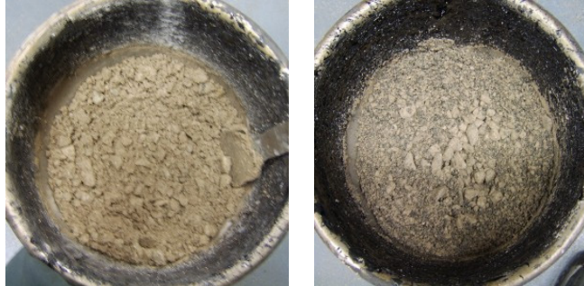
Figure 10. Appearance of wet loose materials; (left) before foaming, (right) after foaming
