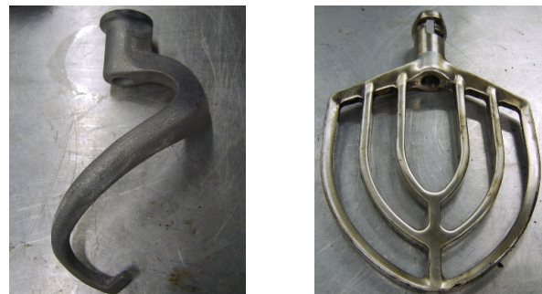
Figure 9. Two types of agitator used in this study, Left: Spiral dough hook type; Right: Flat type
