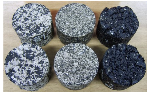
Figure 12. Appearance of compacted specimens; (left) foamed asphalt mixed using spiral dough hook agitator, (middle) foamed asphalt mixed using flat agitator and (right) hot mix asphalt.
