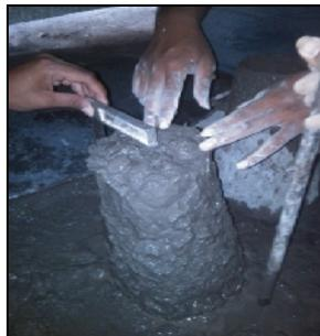
Gambar 1. Hasil *Test slump*
