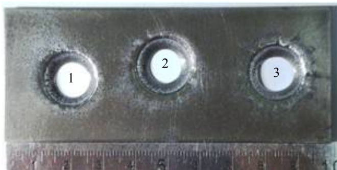
Gambar 5. Contoh hasil drilling ECM hardened toolsteel SKD 11 dimensi 100x40x4,5mm kekerasan >52HRC.
