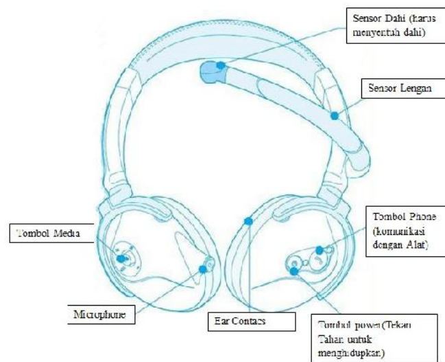
Gambar 1. Sensor MindSet NeuroSky Sumber : Instruction Manual Neurosky Mindset
