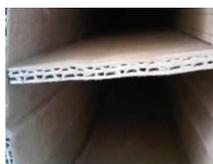
**Gambar 1.** *Double-wall corrugated board flute bc.*
