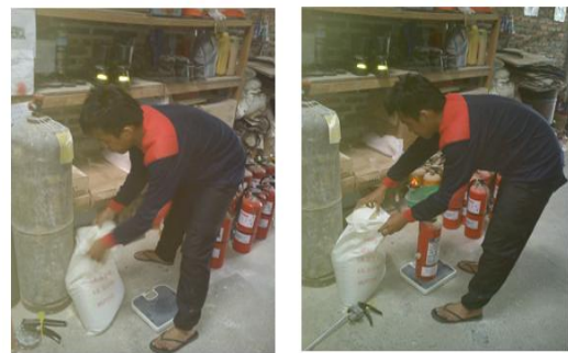
Fig. 1 Initial conditions are charging a fire extinguisher
