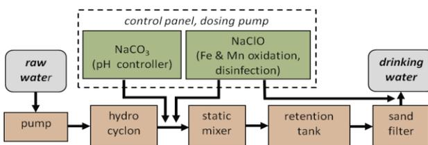
Fig. 4 Water Treatment with chemical solution block diagram
