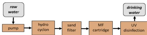
Fig. 6 Water Treatment with cartridge and UV block diagram
