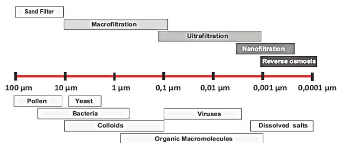
Fig. 1 Water Treatment physical filtration grade [4] (Heijman S.G.J, CT4471, Nanofiltration and Reverse Osmosis, 2007)
