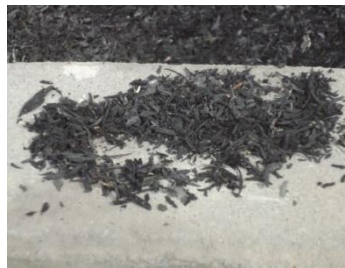
Gambar 3. Karet serutan ( shredded rubber ) hasil vulkanisir ban
