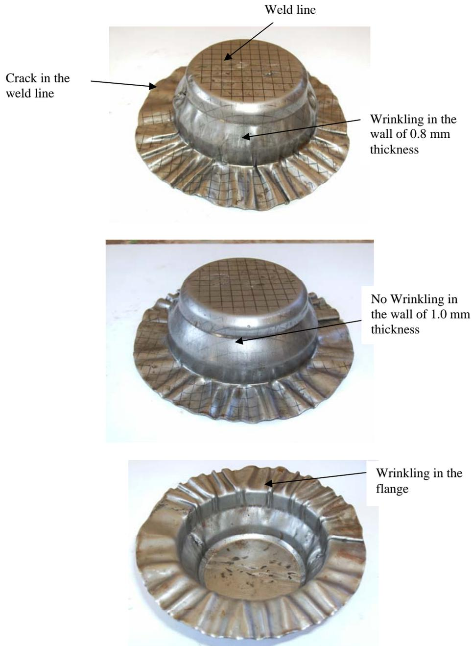
Fig. 5 Drawn parts of tailored welded blank
