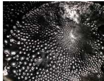
Figure 2 Appearance of the collapsed foamed bitumen
