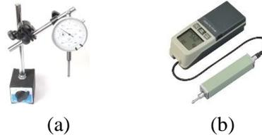
**Gambar 4. (a) Dial indicator, (b) Surface roughness tester**
