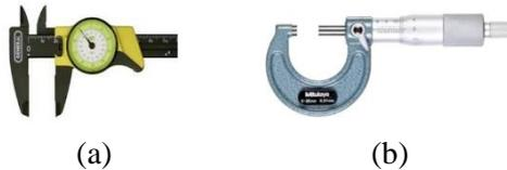
**Gambar 3. (a) Jangka sorong, (b) Outside micrometer**
