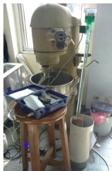
Gambar 2: Pengujian matric suction di laboratorium
