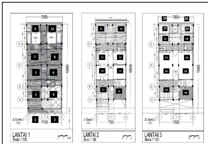
FIGURE 6. The Test Stage (Thursday, September 22 nd , 2016): Testing of Air Temperature, Air Humidity and Wind Speed at 30 Point Locations
