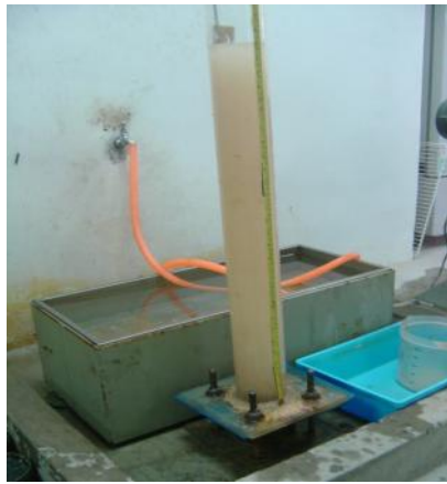
Figure 3. Permeameter for Clogging Test
