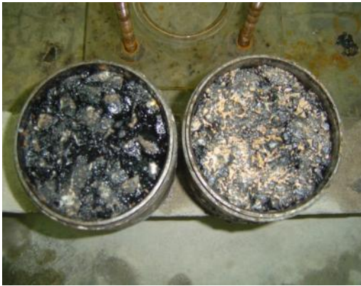
Figure 7. Specimen Condition before and after Clogging by Using Solis
