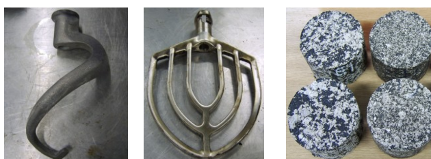
Figure 6. Spiral dough hook (left) and flat (middle) agitator type, and the produced specimens (right)
