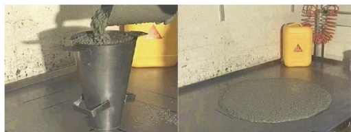
Gambar 1. Pengujian mortar flow test (Prajitno, 2007)
