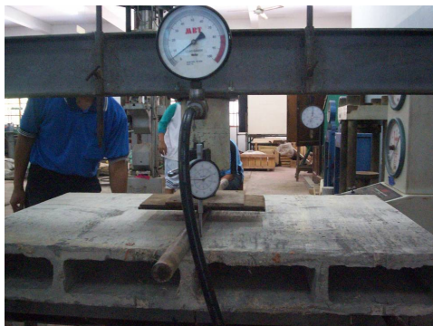
Gambar 7. Pengujian lentur dinding panel type I
