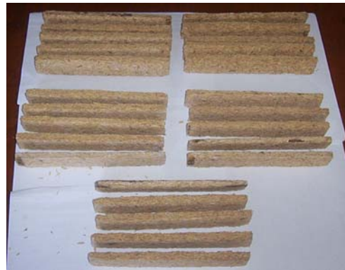
Gambar 41. Spesimen sampel uji bending core SP:UF
