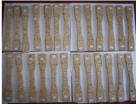
Gambar 38. Spesimen sampel uji tarik core SP:UF
