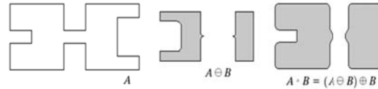
Fig 7. Opening the process used to separate objects as well as to smooth the image
