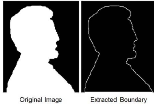
Fig 11. Using a structuring element of 3 x 3 box shape in the process of boundary extraction is obtained images extracted boundary
