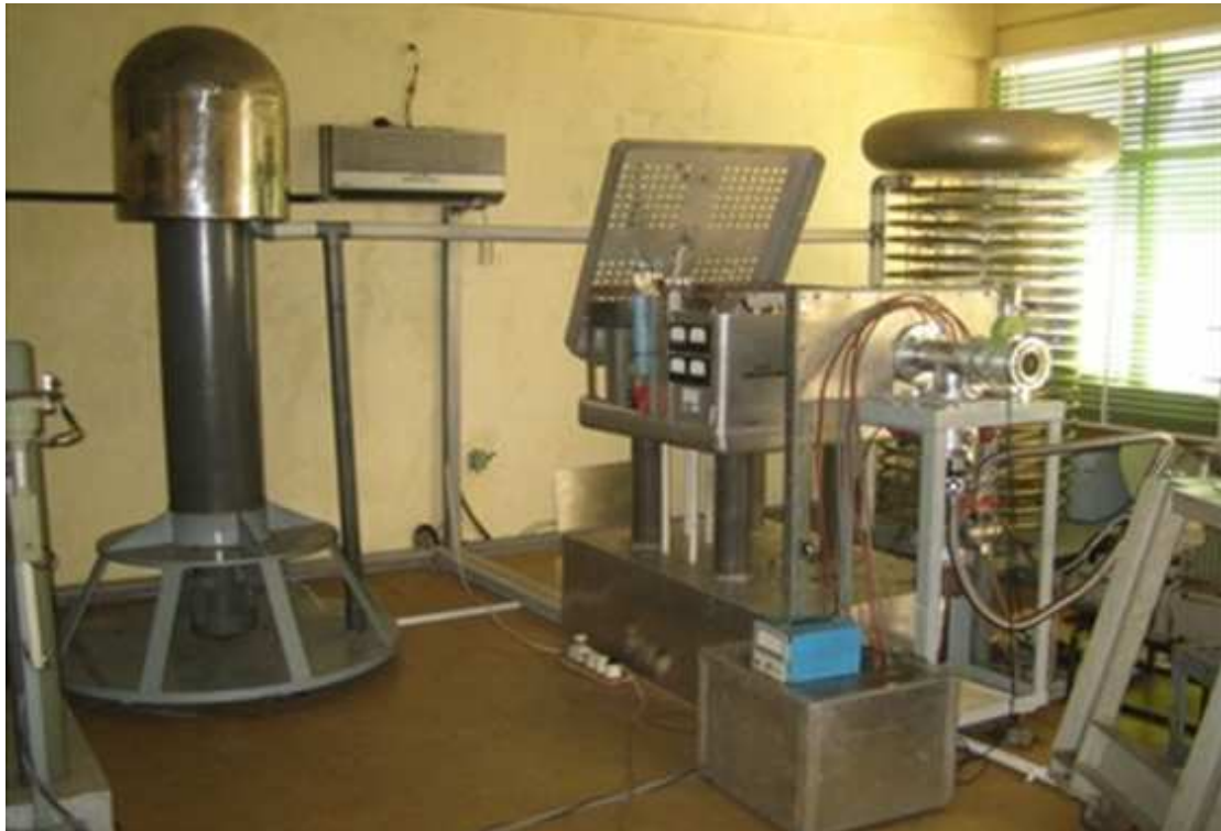
Figure 3: Photograph of the device arrangement for ion implantation
