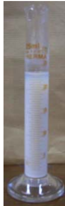
Figure 4. The sample of TiO 2 /distilled water nanofluid.
