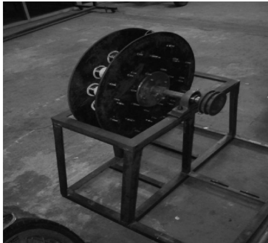
Gambar 2. Generator Magnet Permanen Axial
