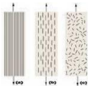
Gambar 2. Skema penyusunan serat (a) continuous fibres , (b) discontinuous fibres , (c) random discontinuous fibres
