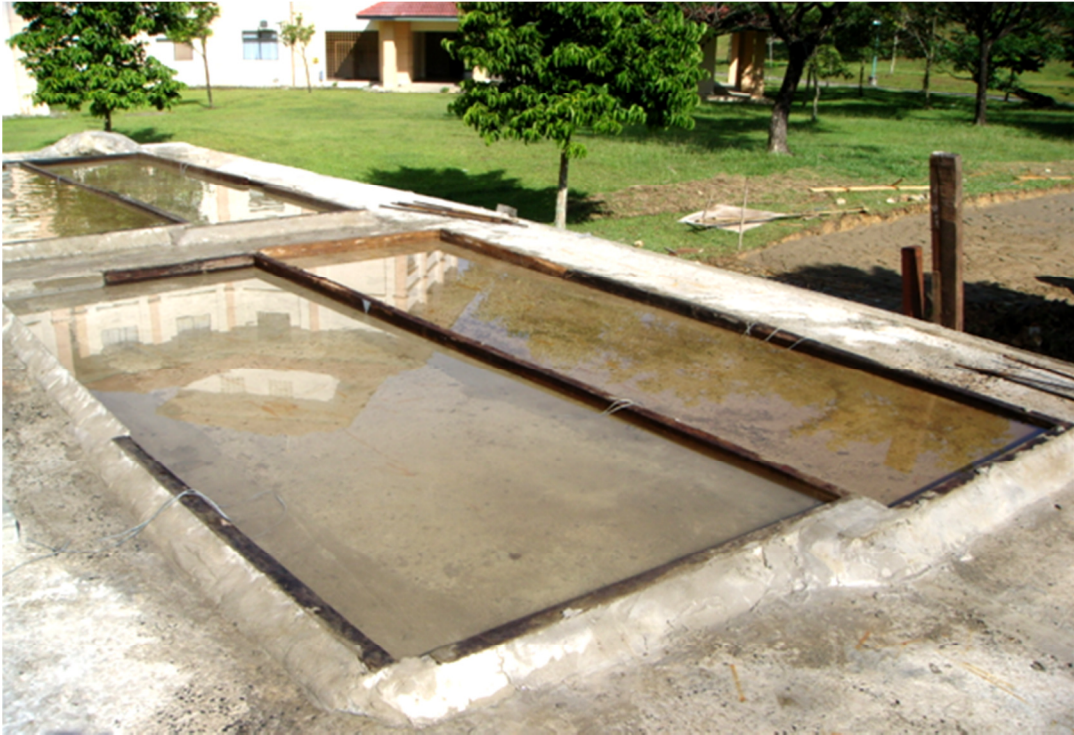
Figure 8: Water ponding with approximate 50 mm deep of water
