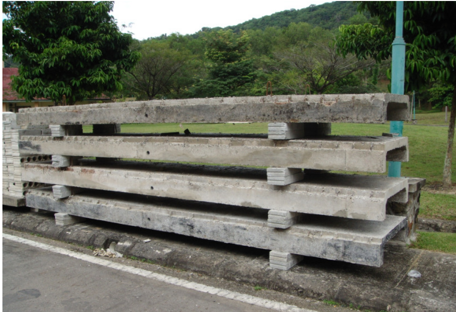
Figure 5: Four units of 5.2 m long C-channels in stacked
