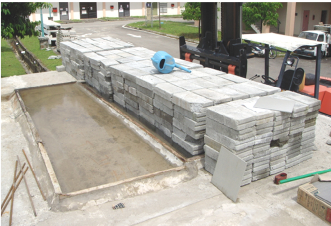
Figure 9: A total load of 10.15 kN/m 2 being placed onto one panel of 5 m x 1 m area
