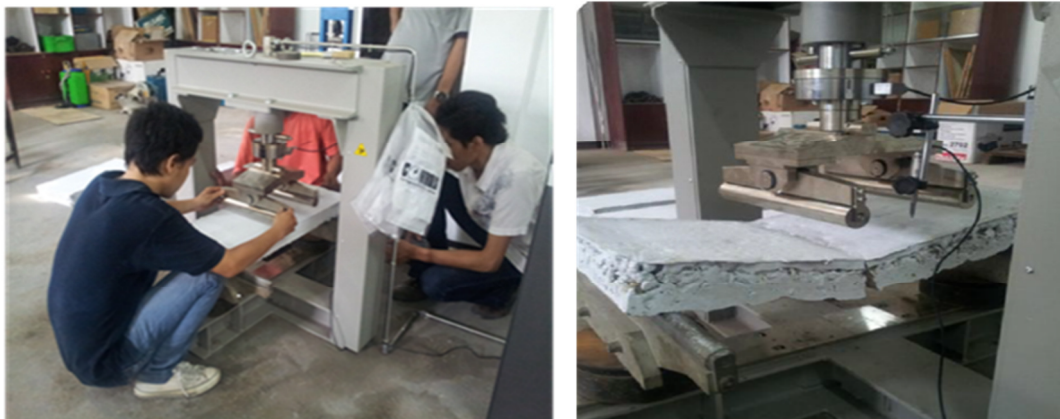
Figure 4 Wall Flexural Test Set-up (left) and the Wall After Testing (right)
