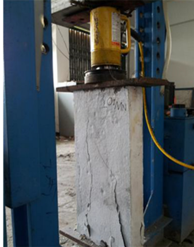
Figure 3 Wall under Axial Compression Test Until Failure
