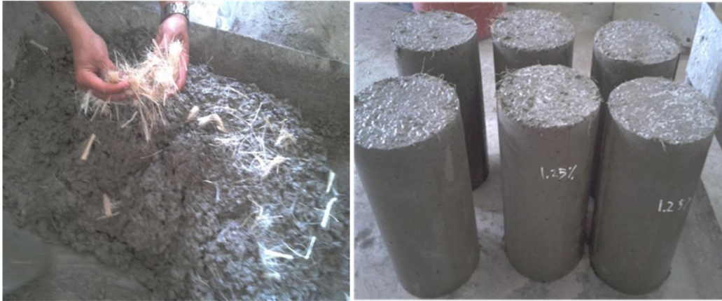
Figure 4. Fibrous Concrete Specimen Preparation
