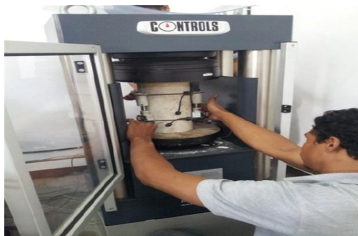
Figure 5. Set-up Compression and Modulus of Elasticity Test
