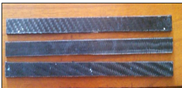
Figure 2. Specimens for modal testing.
