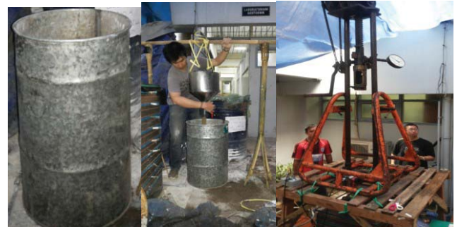
Fig.15. Modeling from sand on “ drum” with Dr 15, 40 % With CPTu
