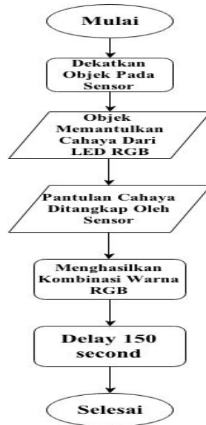
Gambar 2.4. Flowchart Program Kalibrasi Warna
