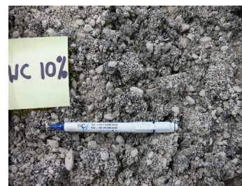
Figure 6. Appearance of binder distribution at 2 seconds mixing time of FAM produced at a FWC of 10%.
