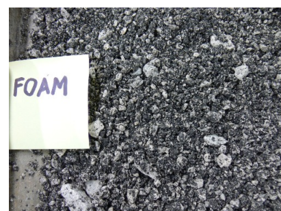
Figure 1. Appearance of binder distribution of hot bitumen sprayed into cold wet aggregates: the mixture is an uncombined asphalt, in which large stiff aggregate-bitumen globules occur.
