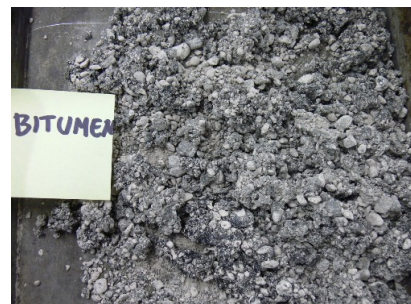
Figure 1. Appearance of binder distribution of hot bitumen sprayed into cold wet aggregates: the mixture is an uncombined asphalt, in which large stiff aggregate-bitumen globules occur.
