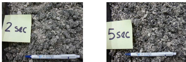
Figure 3. Appearance of binder distribution of FAM at 2 sec mixing time: forming large soft mastic globules and at 5 sec mixing time: forming broken soft mastic globules
