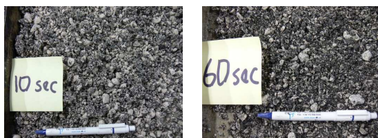
Figure 4. Appearance of binder distribution of FAM at 10 seconds mixing time: forming binder-fines particles and at 60 seconds mixing time: forming small binder-fines particles (well distributed).
