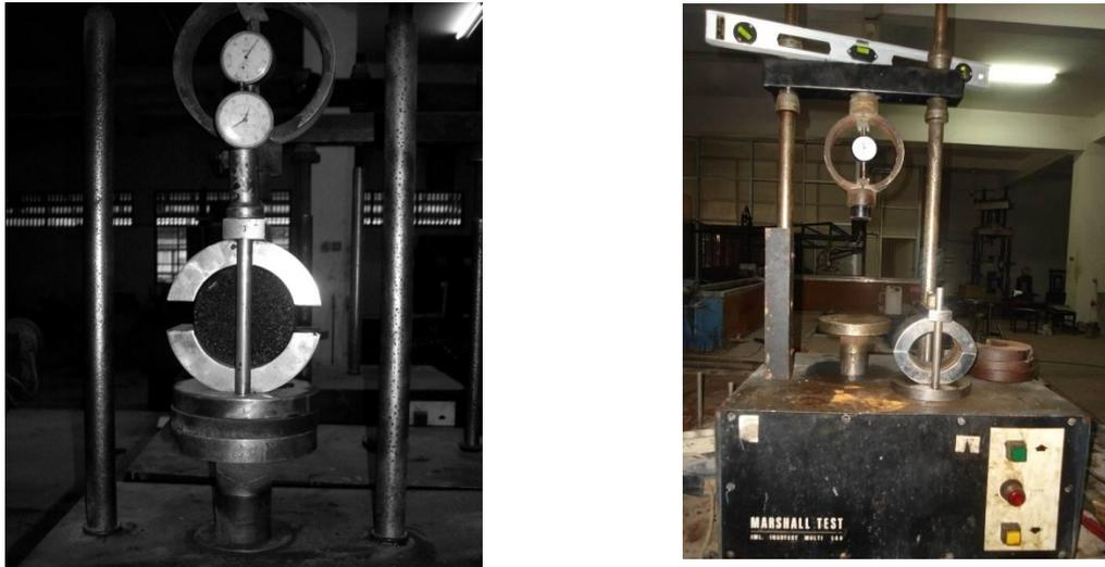
Gambar 1. Alat test *marshall*
