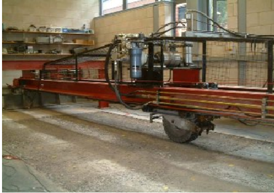
Gambar 1. Alat Pavement Test Facility (PTF) di NTEC
