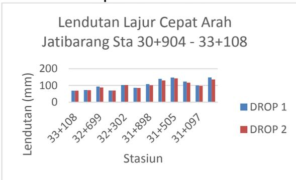
Gambar 4a. Lendutan Sta 30+904 – Sta 33+108 Lajur Cepat Arah Palimanan
