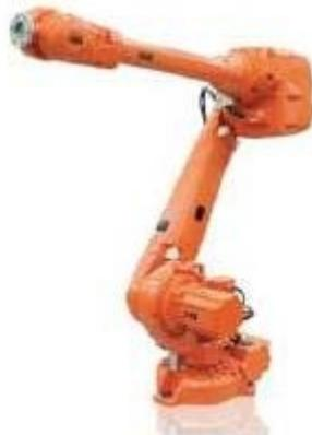
Gambar 4. Robot ABB 6-Axis IRB 4600
