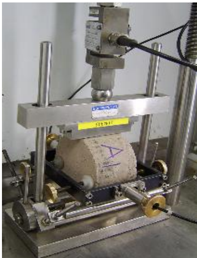
Figure 2. ITSM test configuration
