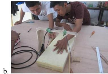
b. Pemotongan *Polyurethane rigid foam*
